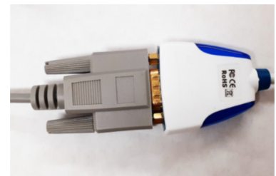
9 Pin Crossover cable attached to RS232 to USB converter.
