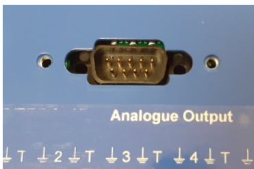
Figura 7. Puerto de terminal RS232 de 9 pines
